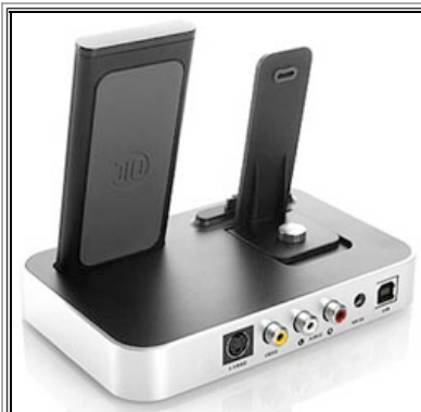
Rear of dock features RCA and S-Video connections.
